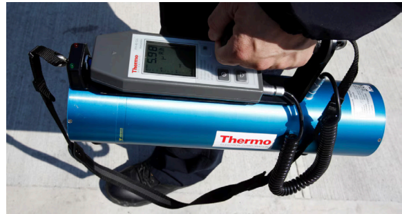
A member of the NYPD holds a device used to detect levels of radiation during a multi-agency "dirty bomb" exercise
